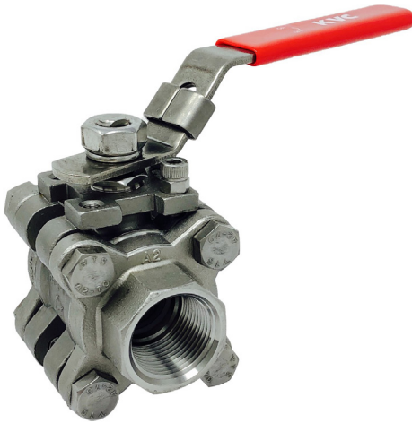
FIG. S-332T: THREADED ENDS, ¼" TO 2": 2000 WOG 2 ½" TO 3":1500 WOG ISO 5211 MOUNTING PAD.
